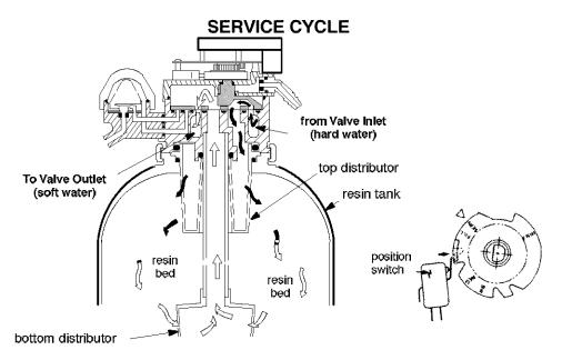
Hard water enters the valve inlet port. Internal valve porting routes the water down and out the top distributor, into the resin tank. Hard water is softened as it passes through the resin bed, then enters the bottom distributor. Soft water flows back into the valve and out the valve outlet, to the house soft water pipes.
